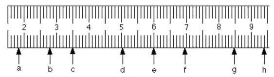
For each of the vernier readings, determine the first two digits from the top scale and the estimated digit from the bottom one: write your answer to the right of each drawing:
